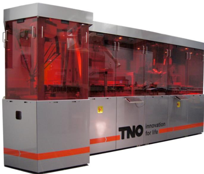
The TNO PrintValley 3D printing setup: a new approach to rapid 3D printing, employing a carousel type-arrangement of building platforms passing underneath multiple printing heads in order to significantly speed up production. The setup can print several dozens of ODF size objects per second. This approach may be used for pharma as well in order to reach relevant production volumes.
