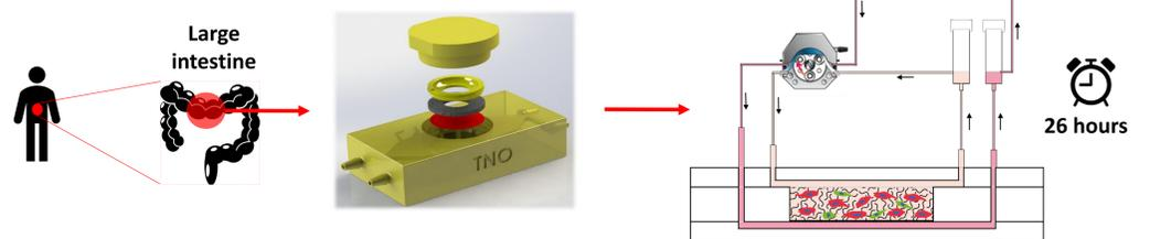
**Fig 2.** Schematic of the experimental design used in this study. We inserted human intestinal tissue (colon) inside the microfluidic chip, maintained it by constant perfusion for 26 hours at two different flow rates (2 and 20 ml/hr).
