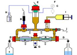
A: peristaltic compartments; B: pH electrode; C: alkali pump; D: filtrate liquid circuit with hollow fibers; E: level sensor; F: N2 gas inlet; G: sampling port; H: gas outlet; I: « ileum effluent » container; J: temperature sensor.
