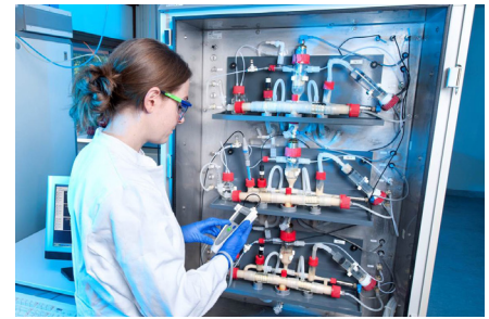
Cabinet with three separate TIM-2 systems simulating the colon.
