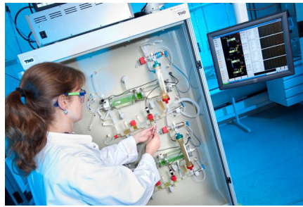
Cabinet with two separate tiny-TIM systems for parallel experiments.
