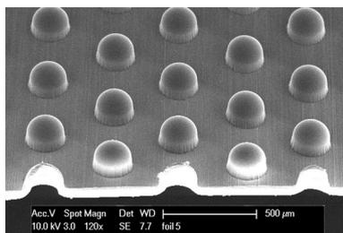
Thermoformed scaffolds in polycarbonate
